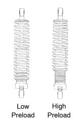
same. When decreasing preload, make sure at least two turns of preload are holding the spring between the retainer on top of the shock and the threaded spring preload adjuster nut on the shock body.
